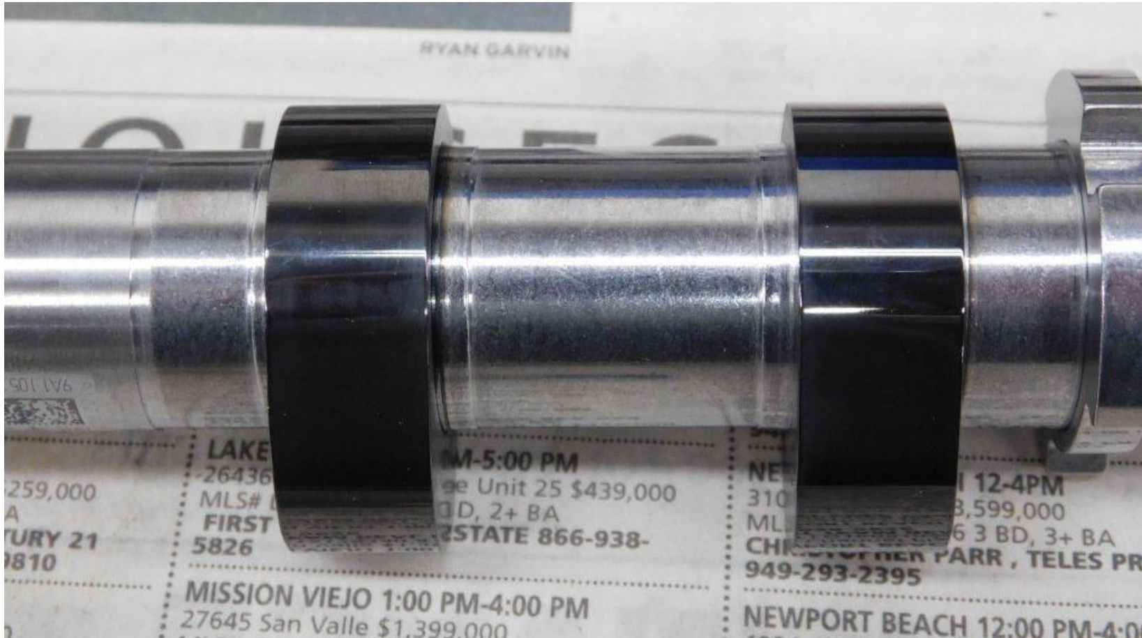
DLC Coating on a cam shaft
